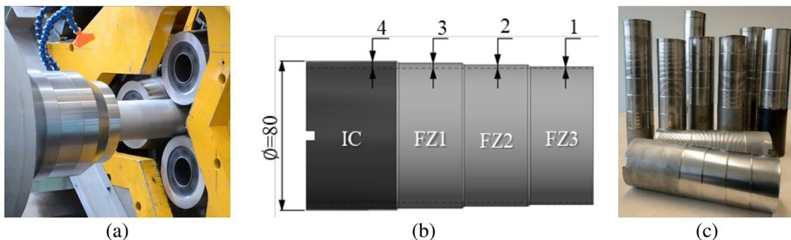
Figure 1. Specimen manufacture: (a) Flow forming machine; (b) geometry and dimensions (in mm), (c) final workpieces.
