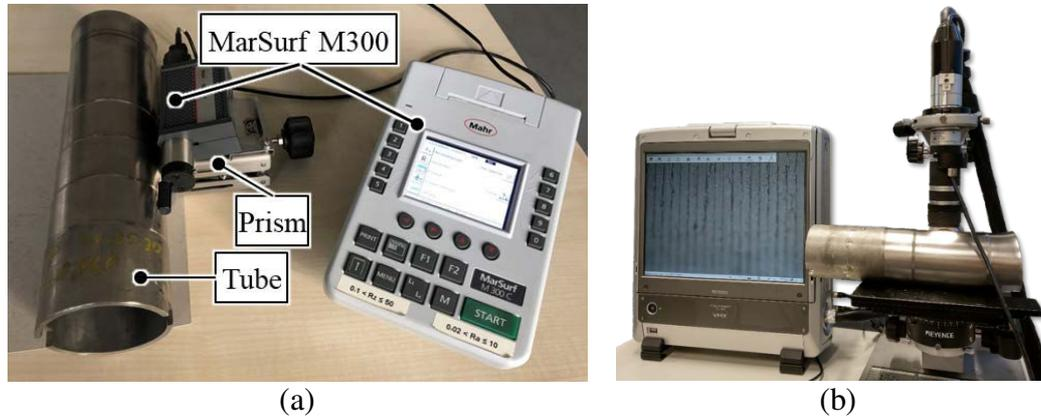
Figure 2. (a) Roughness measurements with the MarSurf M300 and (b) microscopic inspection of the surface with the Keyence VHX-500F.
