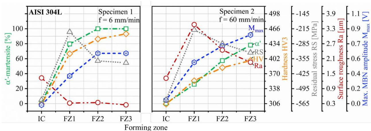
Figure 5. Results of the correlations between non-destructive testing by means of MBN and microstructural phenomena like hardening, residual stresses and roughness, during plastic deformation of austenitic steel AISI 304L.
