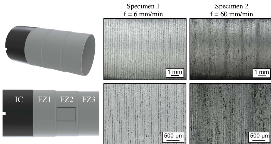
Figure 4. Microscopic investigation of the surface condition of specimens produced using different feed rates.
