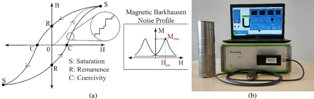
Figure 3. Micromagnetic testing: (a) Hysteresis loop and MBN profile; (b) 3MA-II system device and flow-formed specimen.
