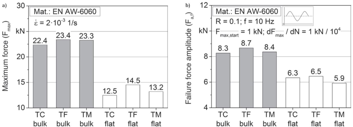
Figure 5: a) Maximum forces in tensile tests, b) failure force amplitudes in load increase tests
