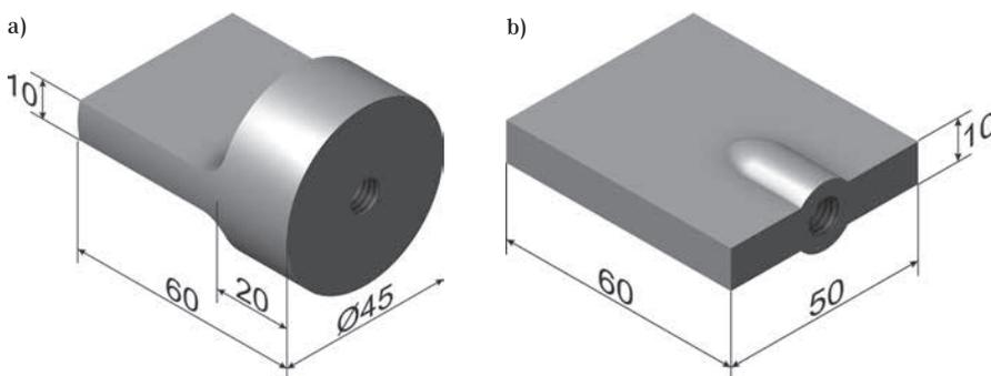
Figure 1: Geometry of specimens, a) bulk material, b) flat profile
