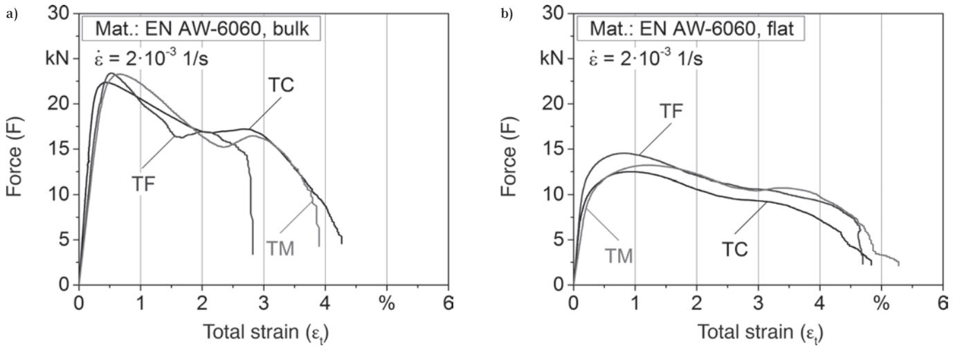
Figure 4: Force-total strain diagrams, a) bulk material, b) flat profile
