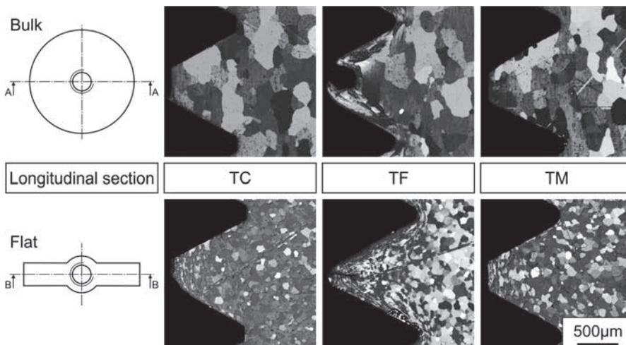
Figure 10: Microstructures of internal threads in bulk material and flat profile specimens at initial condition
