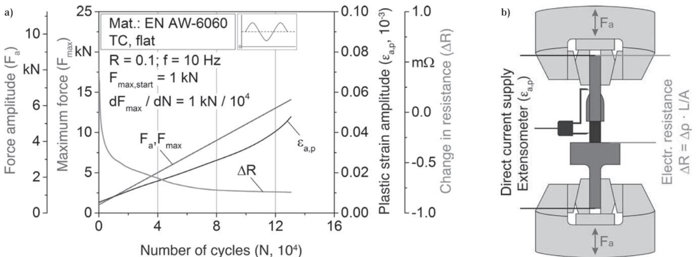
Figure 6: a) Plastic strain amplitude and change in electrical resistance in continuous load increase test for a cut internal thread (TC) in flat profile specimen, b) schematic illustration of clamped flat profile specimen with applied sensors
