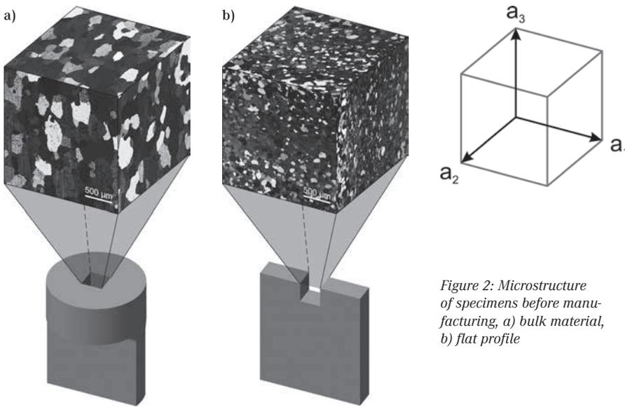
Figure 2: Microstructure of specimens before manufacturing, a) bulk material, b) flat profile
