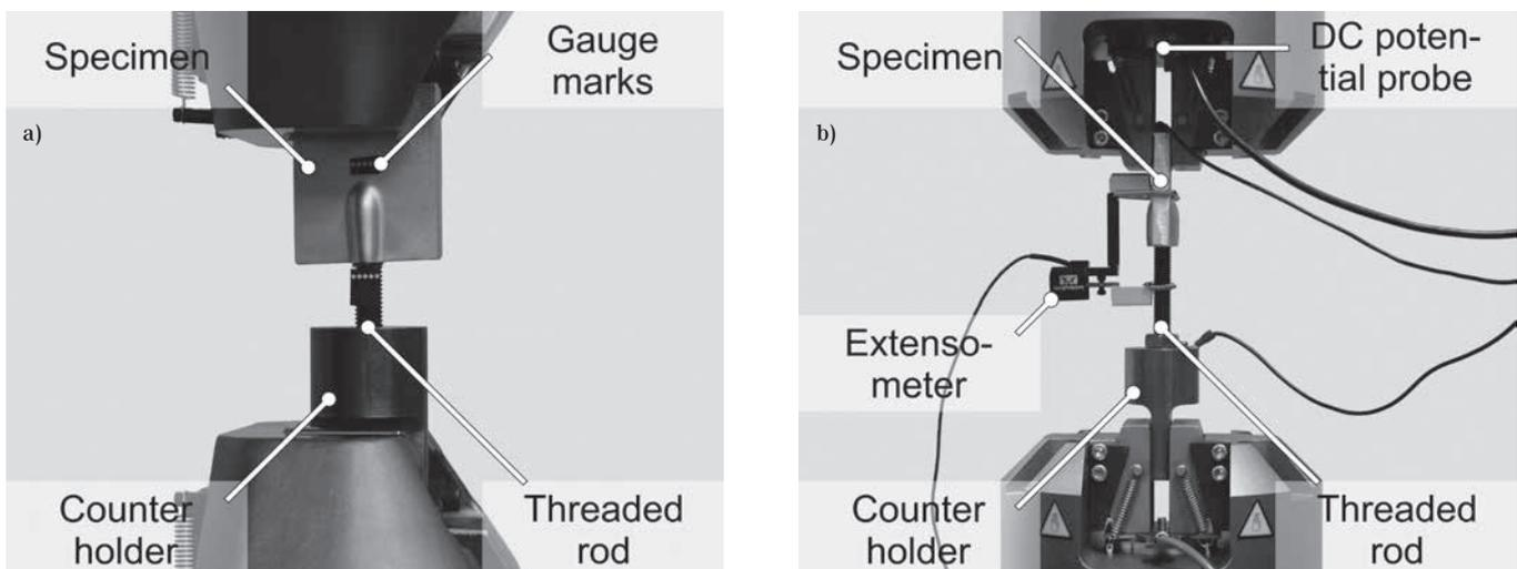
Figure 3: Experimental setups with integrated flat profile specimen, a) tensile test, b) fatigue test
