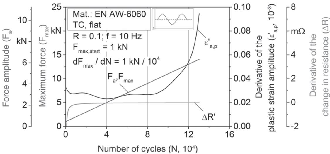
Figure 7: Evaluation of the material reactions for a cut internal thread (TC) in flat profile specimen by means of derivatives
