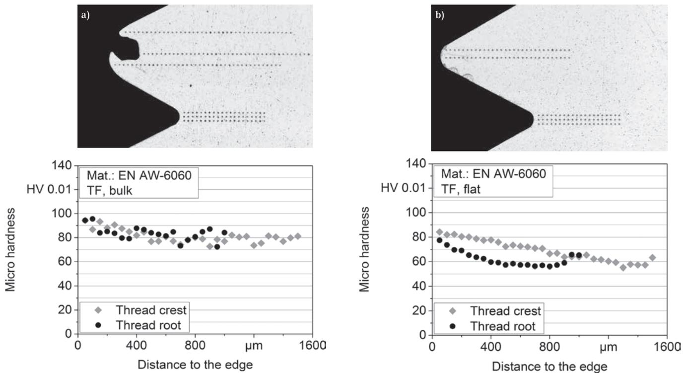
Figure 11: Micro-hardness profiles in thread crests and roots of formed internal threads (TF) a) bulk material, b) flat profile
