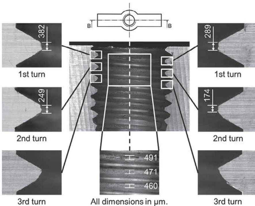
Figure 9: Measuring of thread crests to determine the profile quality of a cut internal thread (TC) in flat profile specimen
