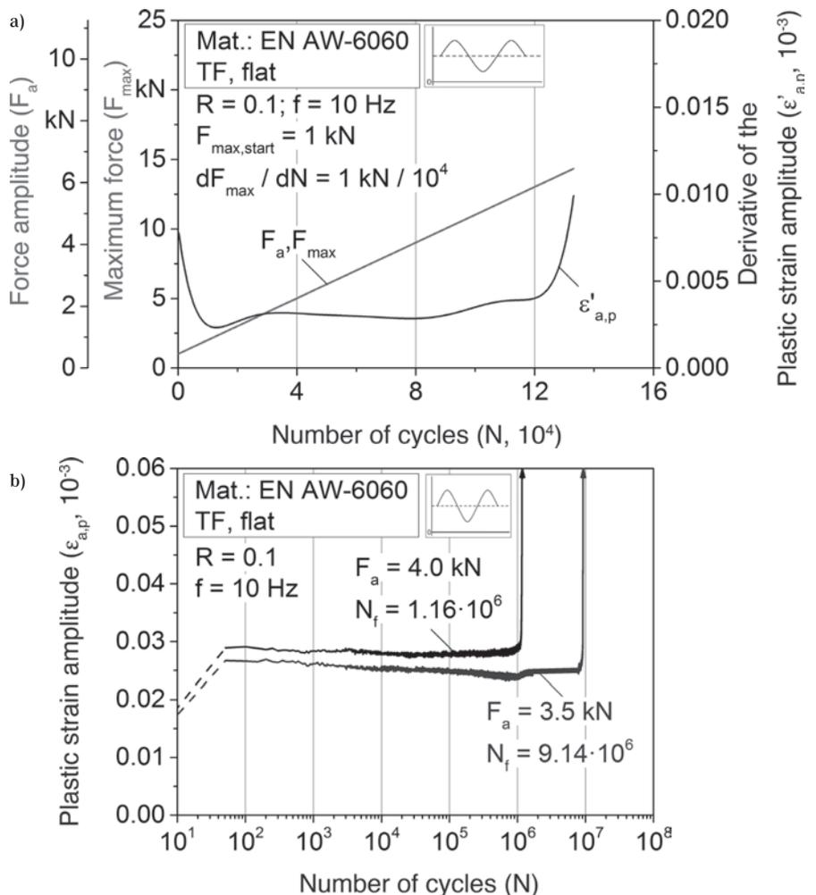
Figure 8: a) Derivative of plastic strain amplitude in continuous load increase test, b) cyclic deformation curves for single step tests; formed internal threads (TF) in flat profile specimens
