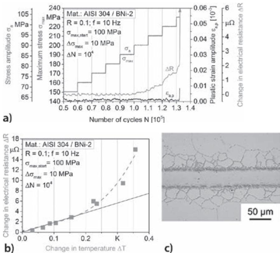
Figure 3. Test results for the AISI 304/BNi-2 brazing joints, a) stepwise load increase test with loading and material reaction values, b) correlation of deformation-induced changes in resistance and temperature, c) microstructural cross-section
