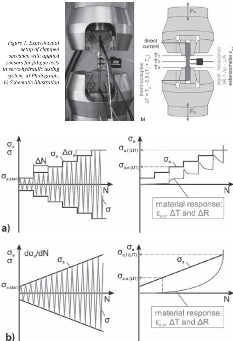
Figure 1. Experimental setup of clamped specimen with applied sensors for fatigue tests in servo-hydraulic testing system, a) Photograph, b) Schematic illustration
