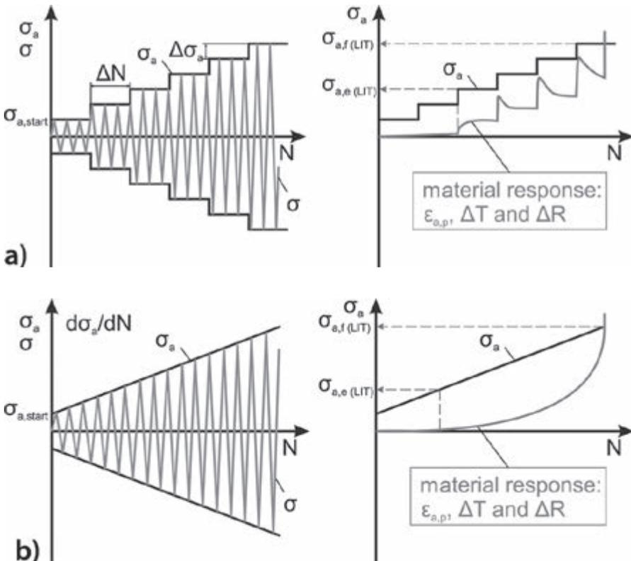
Figure 2. Tests with corresponding material responses as basis for determination of characteristic values, a) stepwise load increase, b) continuous load increase
