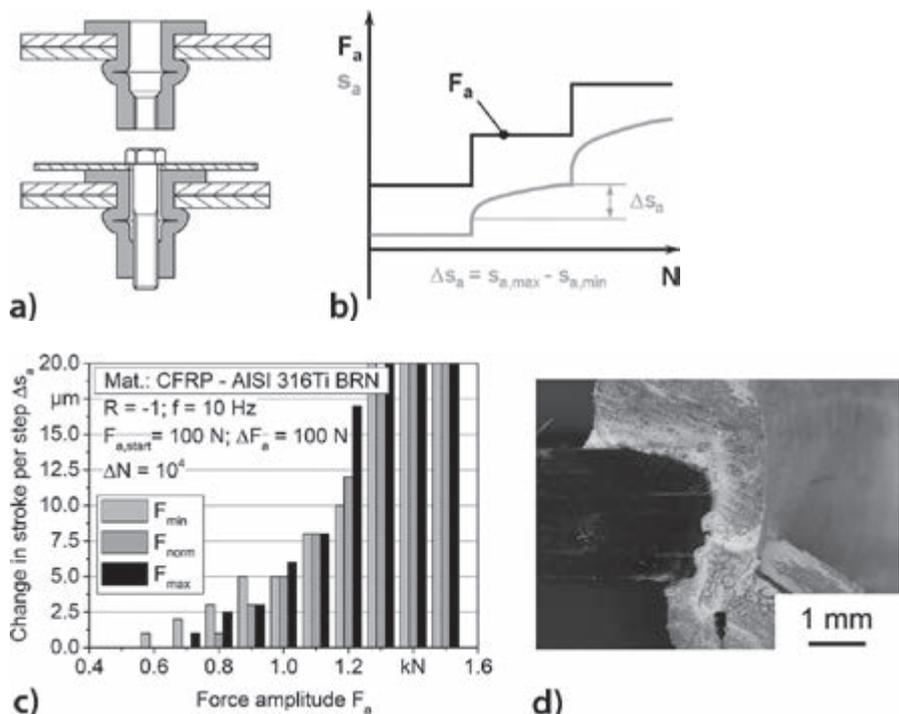
Figure 4. a) Schematic illustration of blind rivet nut compound, b) schematic illustration of stepwise load increase test with measurement of change in displacement, c) change in displacement force amplitude measurement for different plant forces of a CFRP stainless steel compound, d) microstructural cross-section of a CFRP aluminium compound after corrosion treatment
