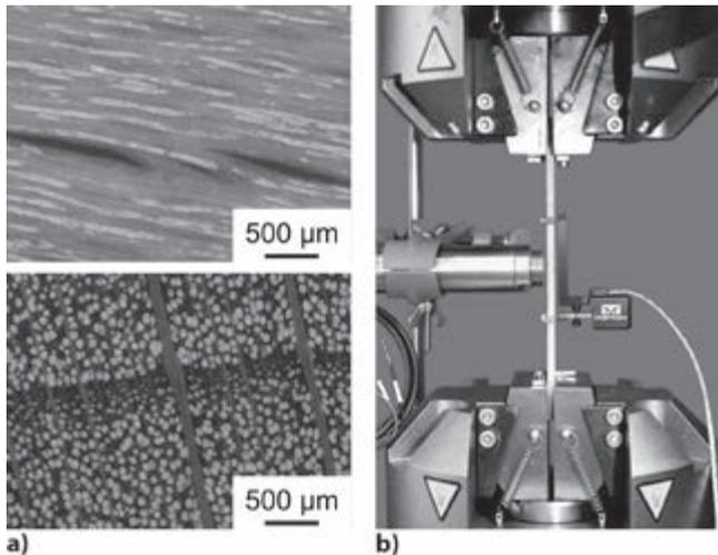
Figure 8. Illustrations for the beech wood tests, a) microstructure in longitudinal (above) and cross-sectional direction (below), b) experimental setup with extensometer (right) and pyrometer (left), c) damage- and fracture-relevant stress amplitudes determined in stepwise load increase test as function of wood fiber direction and for glued joint, d) cyclic deformation curves in single step tests
