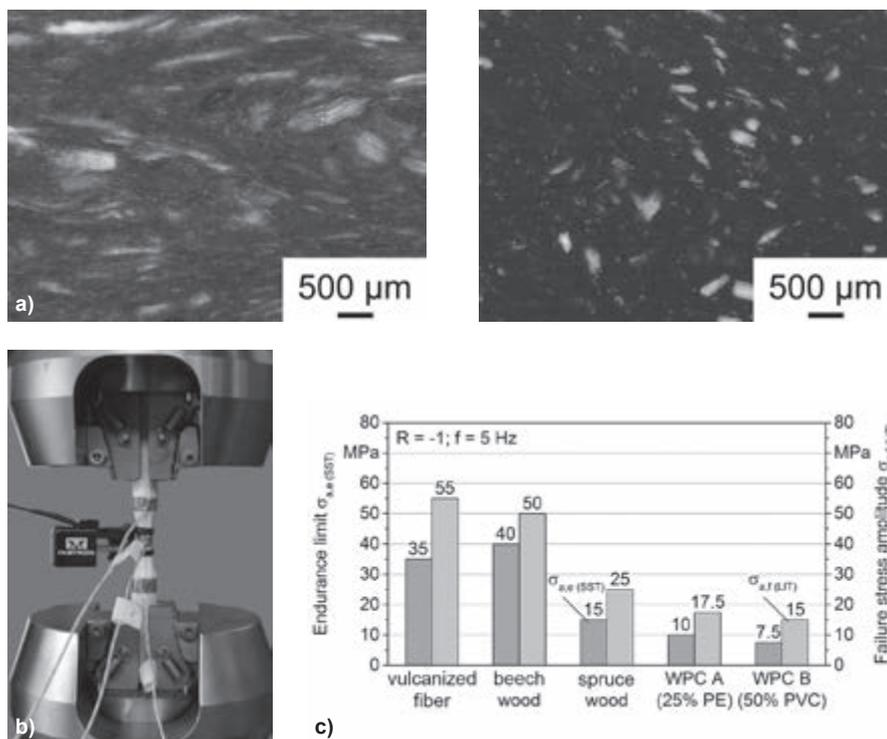
Figure 9. a) Microstructure of 25 % PE WPC (left) and 50 % PVC WPC (right), b) experimental setup with extensometer and thermocouples, c) endurance limits in single step tests and failure stress amplitudes in load increase tests for indicated materials
