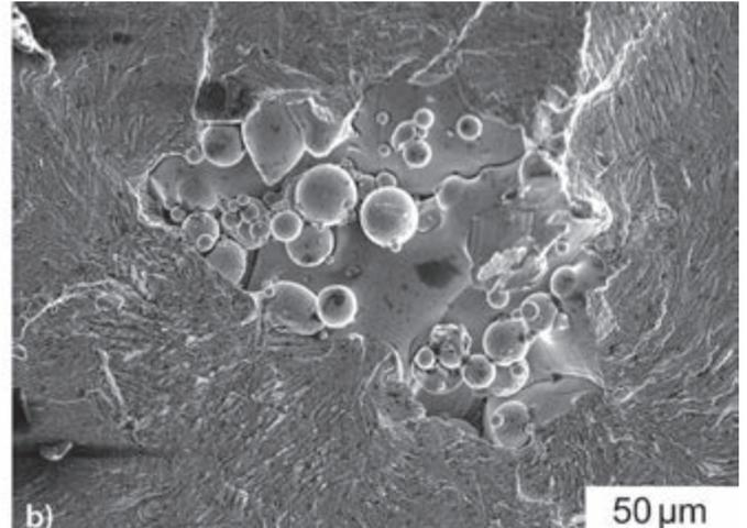
Figure 7. Test results for titanium alloy Ti-6Al-4V, a) Woehler curves for as-built, polished, and shot-peened specimens manufactured by selective laser melting (SLM), b) crack initiation at inner pores
