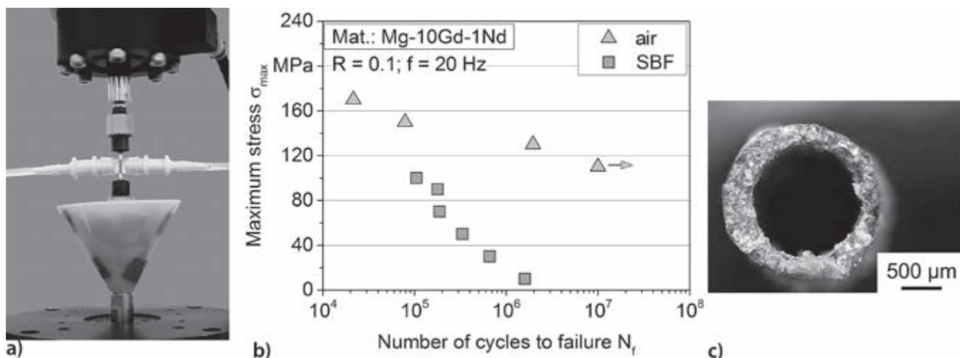
Figure 6. Illustrations for the magnesium stent tubule Mg-10Gd-1Nd, a) Experimental setup for corrosion fatigue tests in micro magnetic fatigue testing system, b) Woehler curves for air at ambient temp. and simulated body fluid at 37 °C, c) fracture surface after fatigue loading in simulated body fluid (SBF) with  $\sigma_{max} = 30$  MPa
