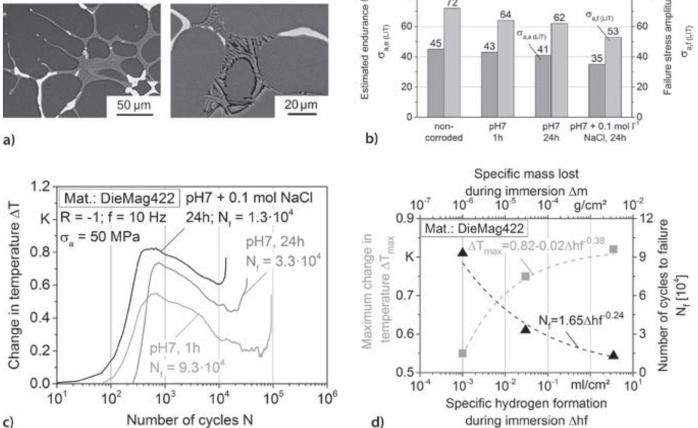
Figure 5. Results for the magnesium alloy DieMag422, a) microstructure in initial state (left) and after corrosion treatment (right), b) estimated endurance limit and determined failure stress amplitudes in continuous load increase tests as function of corrosion state, c) cyclic deformation curves based on change in deformation-induced temperature measurements in single step tests, d) model-based correlation between fatigue and corrosion values
