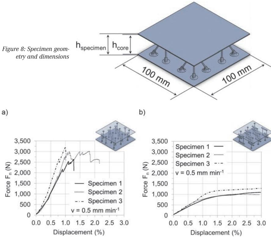
Figure 9: Compression tests with a hexagonal lattice core structure nominal force vs. displacement diagram, a) DIF, b) CLF
