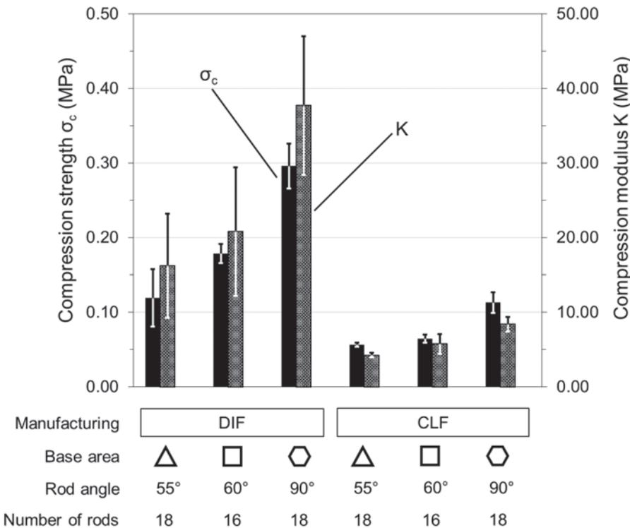
Figure 10: Compression strength  $\sigma_c$  and compression modulus K depending on variation for DIF and CLF
