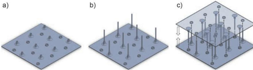
Figure 1: Scheme for differential manufacturing (DIF) process steps, a) individual top layers (FFF), b) manufacturing of lattice core structure, c) manual assembly
